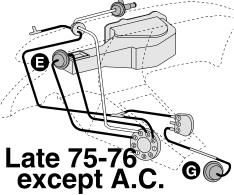
Late 75-76 Heater Vacuum Hose Kit includes 9 color coded vacuum hoses, 2 T-pipe fitting, 18 clamps & a Full Color Schematic Diagram with Instructions. Late 75 does use a hot water valve 9222126 24.50
