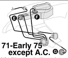
71-Early 75 Heater Vacuum Hose Kit includes 9 color coded vacuum hoses, 2 T-pipe fitting, 18 clamps & a Full Color Schematic Diagram with Instructions. Early 75 does not use a hot water valve 9222124 23.50
