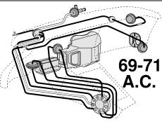
69-71 A.C. Vacuum Hose Kit includes 10 color coded vacuum hoses, 2 T-pipe fitting, 20 clamps & a Full Color Schematic Diagram with Instructions. 9222105 31.95
