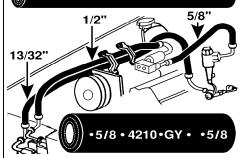
These sets include 13/32", 1/2" and 5/8" O.D. double extruded high pressure freon hoses with 2 internal cloth reinforcements. This is NOT the thinner later model thin wall synthetic hose that lacks inner reinforcements.
