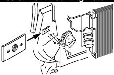
66-67 Horn Mounting Plate on the Fender Skirt Displaced by the condenser & receiver drier, the horns mount to the front inner fender skirt with these plates Complete with bolt, lock washer & 2 OEM Aluminum rivets. 2 read. 9218158 12.50 Ea
