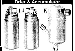
Receiver Dryers & Accumulators remove moisture from the air. **TIP**: examine the sight glass on top of the drier after operating the AC for several minutes. The refrigerant should be clear or may show an occasional bubbles at high temperatures. Lots of bubbles mean the refrigerant is low. Dirt, foam or oil streaks indicates a leak. The desiccant powder in our dryers is compatible with either R12 or R134.
