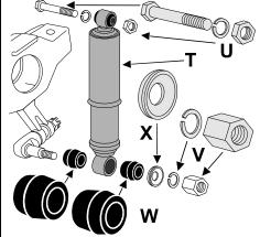
Shock Mounting Hardware One Set does both shocks
