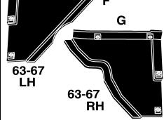
64-68 Inner Large Splash Shields USA64-Early 68 Inner Splash Shield 16 Piece Mounting Kitwith 8 indented hex self tapping bolts with starter pointsplus 8 washers. Does 1 car.81531684.40These mount on the inboard side of the frame railsjust in front of the firewallH64-67 RH Shield All models815316518.75164-67 RH Shield 327 only815316618.75
