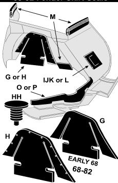
G Early 68 A-Frame Dust Seals Pair. 1 car. Authentic rough textured surface rubber without any mounting holes & longer flaps than late 68-82. Early 68 mounts with staples, so check your inner skirts for evidence of staple holes. 8153142 13.50
