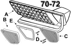
A 70-72 Parking Lamp Housing Includes lamp housing, socket & outer Chrome "honeycomb" grill.
