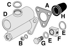
E 53-62 Inner & Outer Copper Crush Washer Set
