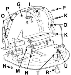
Glove Box Frame To Dash Mtg Hardware
