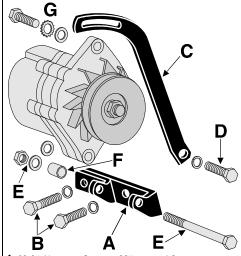
A 63-65 Alternator Support 327 except AC 2277130 34.95 Mounts on exhaust manifold.
