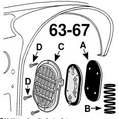
B63-67 Vent Door Pin Spring Pair necessary to mounts the vent doors to door housing. 8844124 C63-67 Fresh Air Vent Door Grills Black plastic
