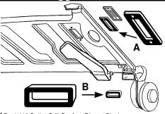
J Deck Lid Outlet Grill Gasket Die cut Black sponge prevents leaks on deck lid. 9778102 KLower To Upper Duct Gasket Die cut poly foam seals the junction of the upper & lower defogger ducts when the deck lid is lowered. 9778104 **5.00**
