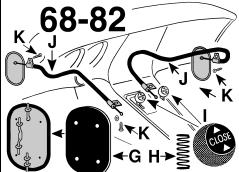
H68-82 Vent Door Pin Spring mounts the vent doors to the vent door housing. Pair 8844124 Knobs: 68-76 Vent Door Control Knob on the Console
