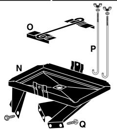
N 63-67 Battery Tray A.C. or 396 2333125 53.50 O 63-67 Retainer with A.C. or 396 Covered with Rubber. 2333126 12.95
