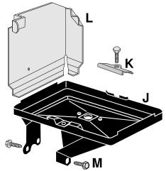
67 Battery Tray except AC 2333130 53.50 Paint as required. 67 Retainer with Mounting Bolt. 2333140 6.50 L 67 Heat Shield except AC 2333132 29.50 Paint as required.
